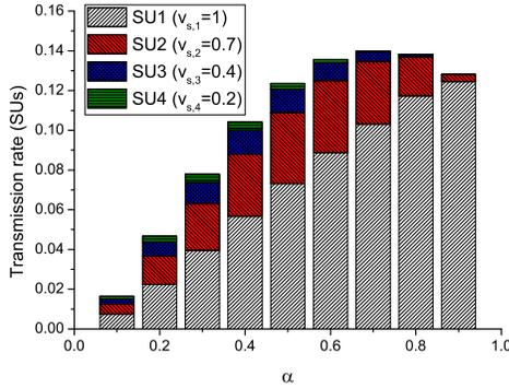
Fig. 6. Simulation with four SUs of different weights  $v_{s,i}$ . It clarifies the trade-off of  $\alpha$  between the throughput and the fairness in the secondary network. Settings around  $\alpha = 0.5$  provide a good balance.
