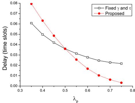
Fig. 4. Average delay of the primary traffic.
