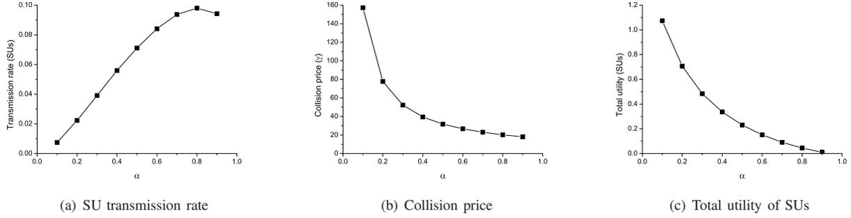
Fig. 5. Sensitivity on  $\alpha$ . The transmission rate of SU linearly increases when  $\alpha$  is small, and the collision price is inversely proportional to  $\alpha$ . The utility of the SU decreases since  $\lambda_{s,i} \leq 1$ .
