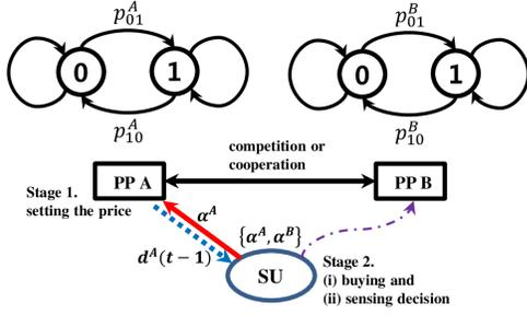
Fig. 1: Channel and game models. PP  $i$  sets price  $\alpha^i$  for the channel information  $d^i(t-1)$ . The SU decides to buy the information, and then, selects the channel to sense. Depending on the sensing result, the SU transmits on the channel that it sensed.
