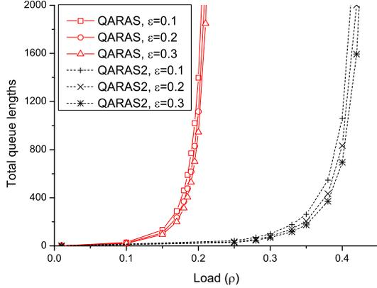
Fig. 2. Performance of QARAS and QARAS2 in a grid network.
