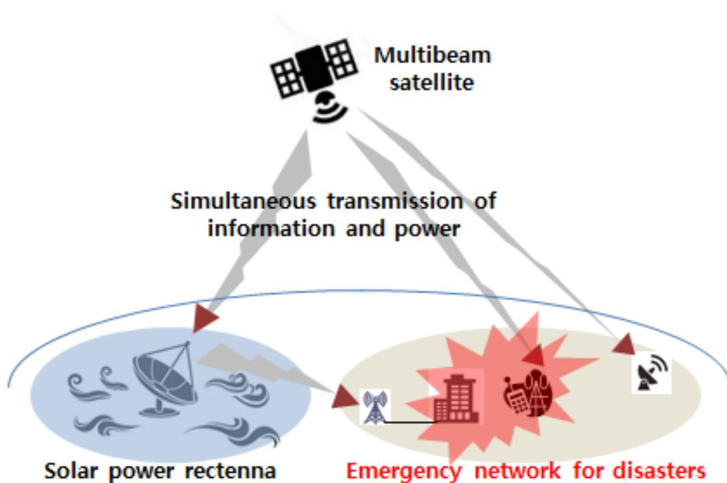
Fig. 1. An emergency network with simultaneous transmission of information and power.
