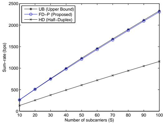
Fig. 1. Performance of UB, PD-P, and HD in symmetric channel when  $N = 50$  and  $D = 500$  m. The sum-rate of each scheme linearly increases with the number of subcarriers  $S$  due to the growing bandwidth. The performance gap between UB and FD-P is negligible, showing that FD-P achieves near-optimal performance.
