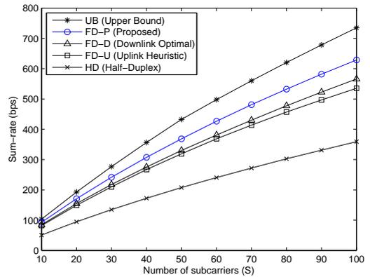
Fig. 3. Performance comparison in asymmetric channel environments when  $N = 50$  and  $D = 500$  m. FD-P outperforms FD-D and FD-U with a gain of 9.7% to 11.1% and 13.6% to 17.4%, respectively.
