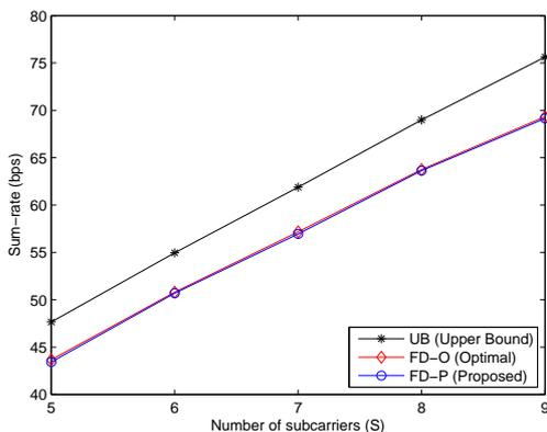
Fig. 2. Performance comparison in asymmetric channel environments when  $N = 5$  and  $D = 500$  m. FD-P achieves almost the same performance with FD-O, and thus it is empirically near-optimal.
