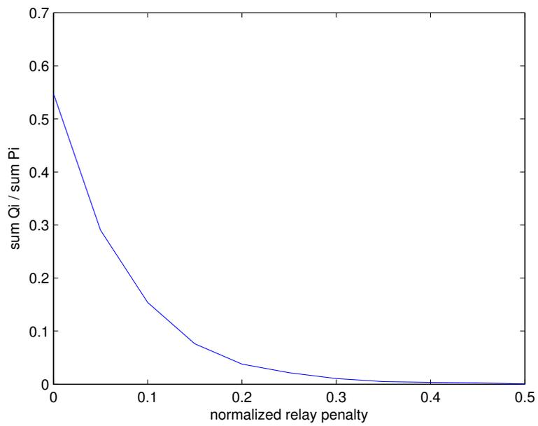
Figure 3. Ratio of power allocation to the ground relay and direct transmission as a function of normalized relay penalty.
