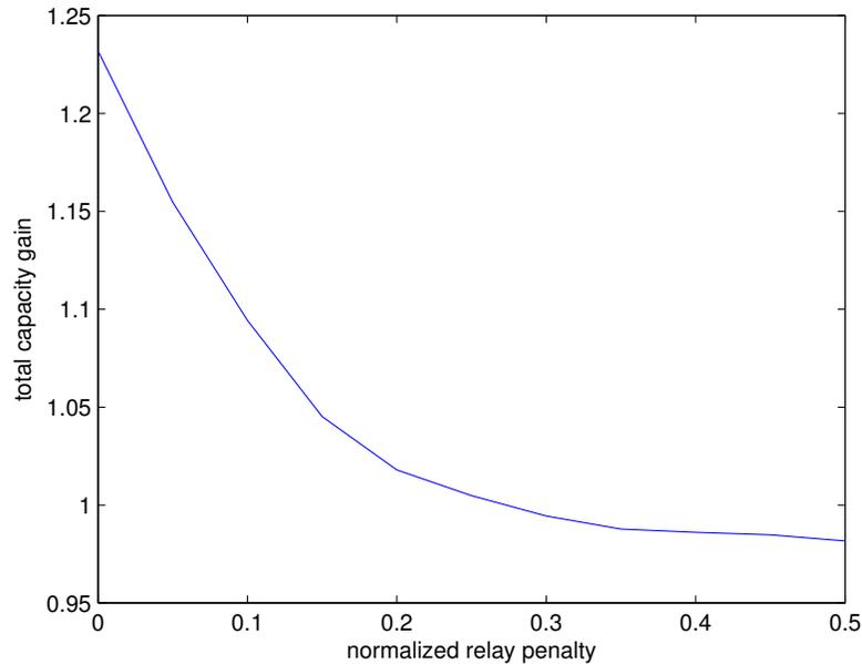
**Figure 2.** Sum capacity gain of using a ground relay, compared to not using, as a function of normalized relay penalty.
