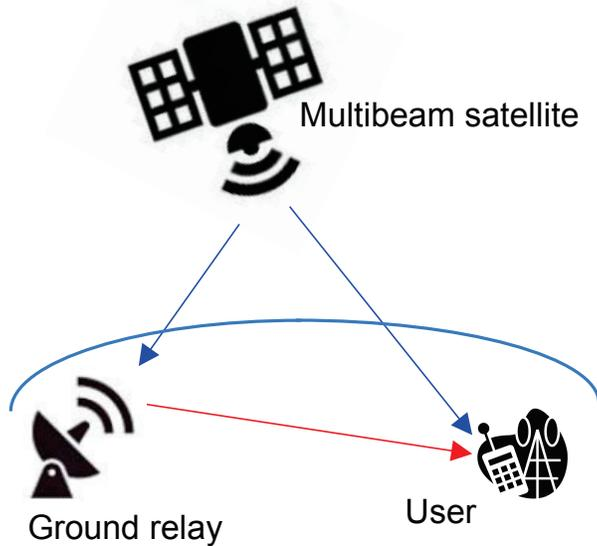
Figure 1. A simple space-terrestrial heterogeneous network with a multibeam satellite and a ground relay on the Earth.
