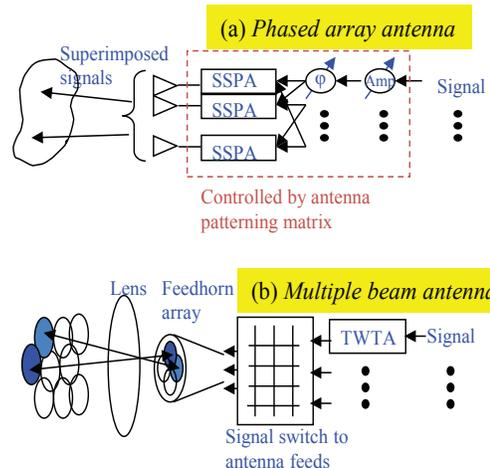
Fig. 2. Schematics of (a) phased array antenna and (b) multiple beam antenna
