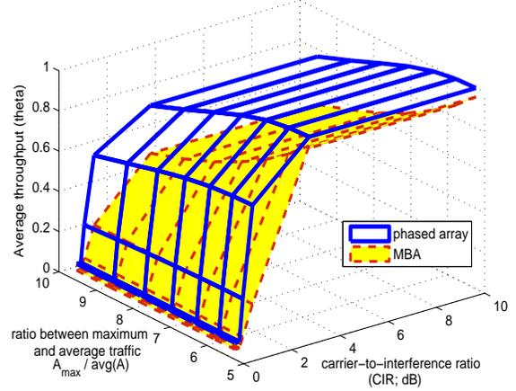
Fig. 5. Steady-state throughput performance comparison of the phased array antenna and the multiple beam antenna as a function of traffic distribution and CIR
