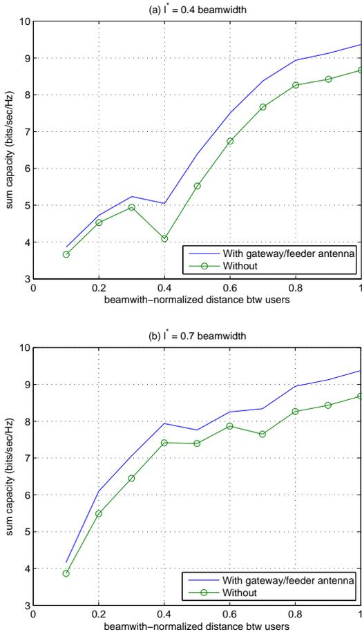
Fig. 6. Comparison of the sum capacities with and without the use of gateway/feeder antenna: (a)  $l^* = 0.4 \frac{\lambda L}{D}$  (b)  $l^* = 0.7 \frac{\lambda L}{D}$
