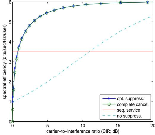
Fig. 3. Capacity of one user as a function of CIR at the SNR of 10.2 dB
