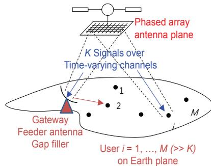
Fig. 1. A multibeam satellite with  $K$  active spotbeams and a gateway/feeder antenna/gap filler on the Earth, to serve  $M$  users
