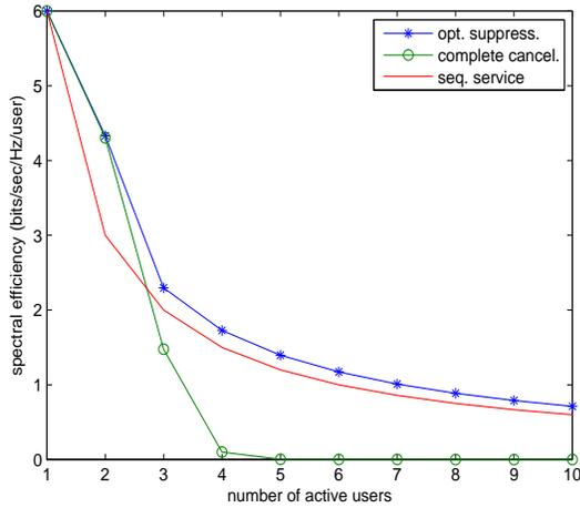
Fig. 4. Capacity of one user as a function of the number of active users within one beamwidth at the SNR of 10.2 dB
