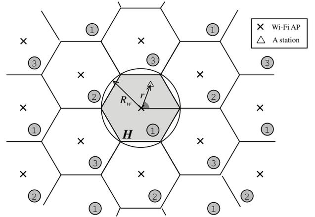
Fig. 5. Hexagonally-deployed Wi-Fi APs with radius  $R_w$  (Super Wi-Fi APs are similarly deployed with  $R_s$ ).
